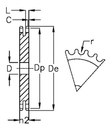
C = 2 D = 25 De = 276.5 Dp = 267.03 For chain size =  $3/4 \times 7/16$ For chain type = 12 B-2 h2 = 30.3 L = 10.8 Number of teeth = 44r = 12.07
